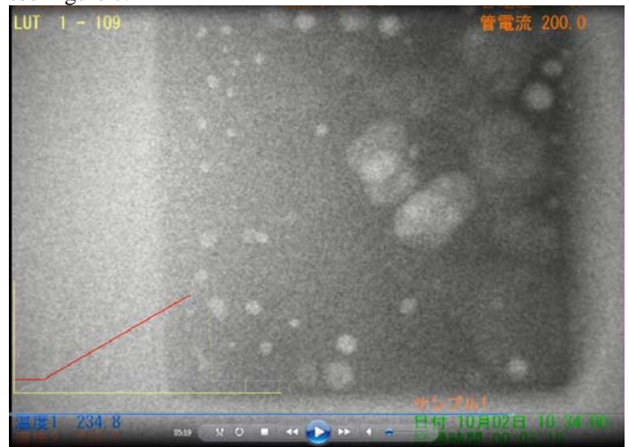
Figure 7. Large Voids Photographed as Solder Reaches Liquidus
