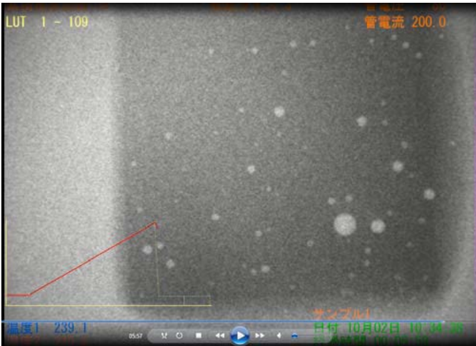
Figure 8. Reduced Voiding After Extended Time Above Liquidus
