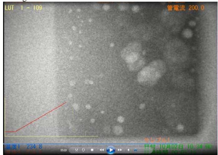
Figure 7. Large Voids Photographed as Solder Reaches Liquidus
